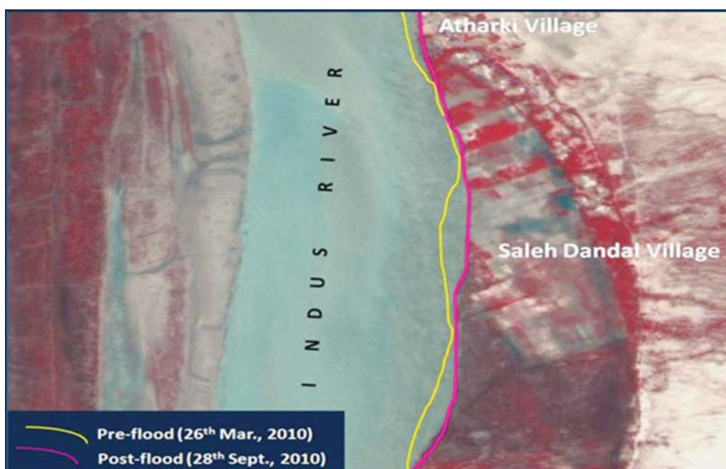
Figure 8: Erosion due to flood 2010 along Indus River, In Atharki Village.
